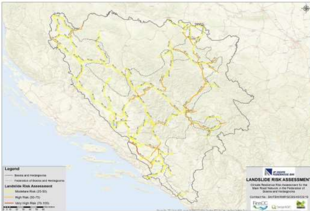
Figure 50: Risk assessment map for landslides
