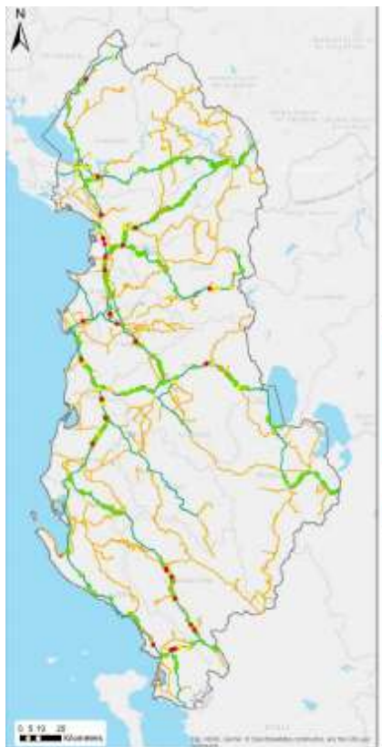
Figure 43: Amount of damages from pluvial floods t=50 due to insufficient capacity of bridges and largest culverts
